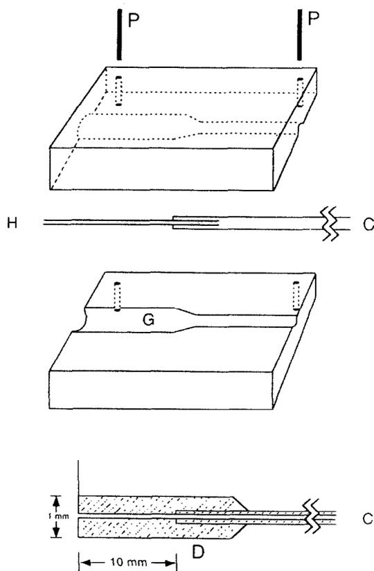
Fig. 7. Preparation of dialysis tubing (D) attached to the capillary (C). G, groove; H, single hair; P, guide pins.
